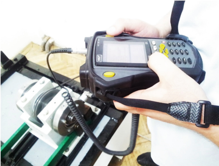
Fig. 3. Sample bearings vibration measurements using the measurement instrument SKF Microlog Analyzer GX [17].
