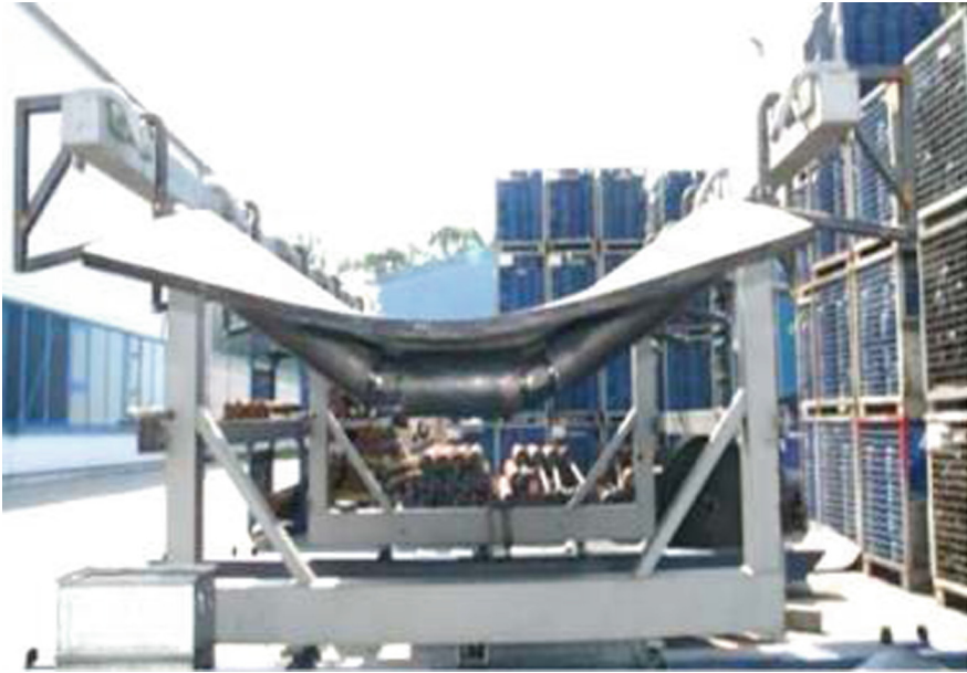
Fig. 7. Contact between unloaded belt and wing conveyor idlers
