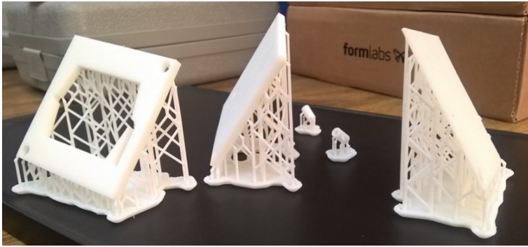
Fig. 8. SLA print of PEM fuel cell reformer.
